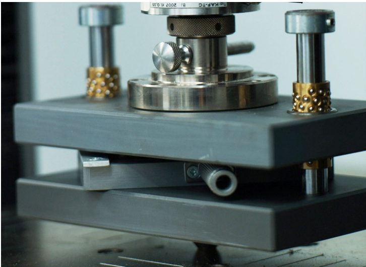
Holder placed between the platens in a compressive tester
