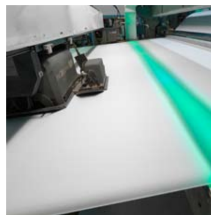
HIGH TECHNOLOGY SCAN. PM7 at Skärblacka has been equipped with, among other things, a hole and spot detector, which digitally scans the paper before it is wound onto a reel.
